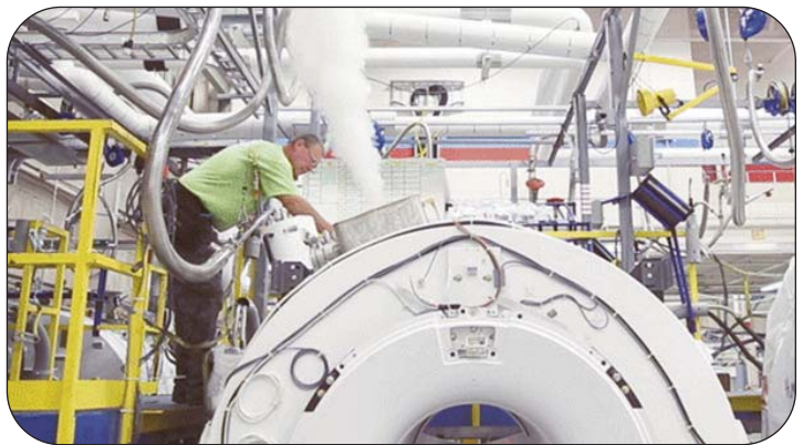
Thorburn's Met-O-Seal Series MTS4 hose coupling used for loading liquid helium in an MRI machine at -269°C (-452°F) just above absolute zero. Magnets at that temperature lose all electrical resistance and become superconducting thus produce the same magnetic field for a thousand years with no more power required.
