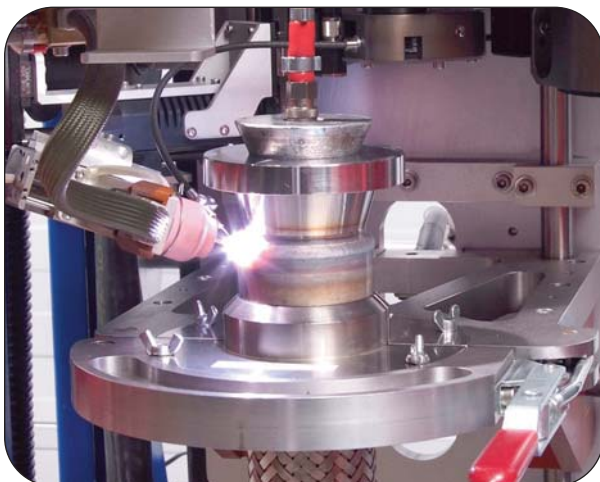
Automated fitting to end joint orbital welding
