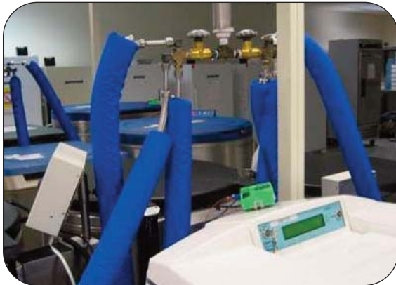
If the room temperature hose consumes 25 liters with an average fill, the consumption of the same hose with CryoTherm™ will be one tenth of this, 2.5 liters loss per average fill
