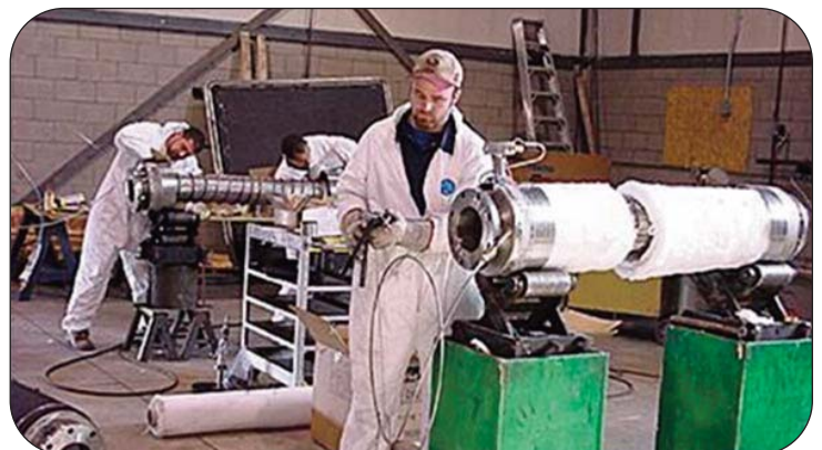
Thorburn technicians assembling Sure-Temp electrically heated hose assemblies
