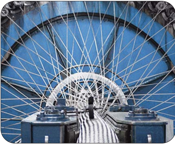
Thorburn uses a range of braiding machines (24, 36, 48, 64, 96 & 128 carriers), with the ability to produce top quality braid from 6mm (1/4") to 350mm (14") nominal size diameter.
